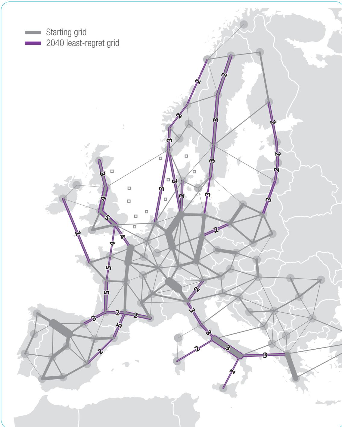
Figure 18: Grid architecture for 2040, robust to the five scenarios (grey: starting grid; purple: reinforcements)
