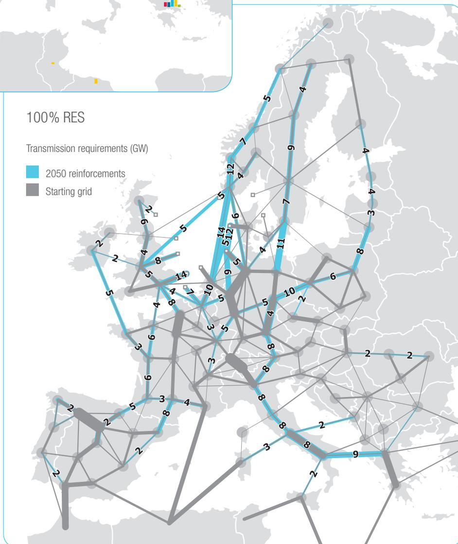
Figure 12 D: Transmission requirements identified in scenario 100% RES (GW)
