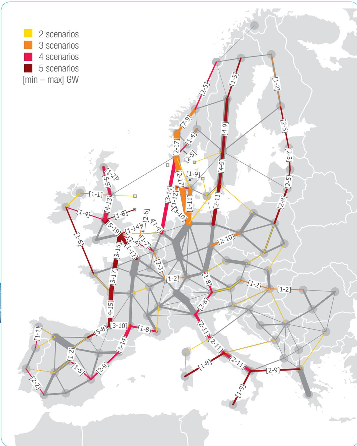
Figure 14: Common reinforcements (widths are according to average reinforcement capacity and the colour represents the number of scenarios where the reinforcement is needed)
