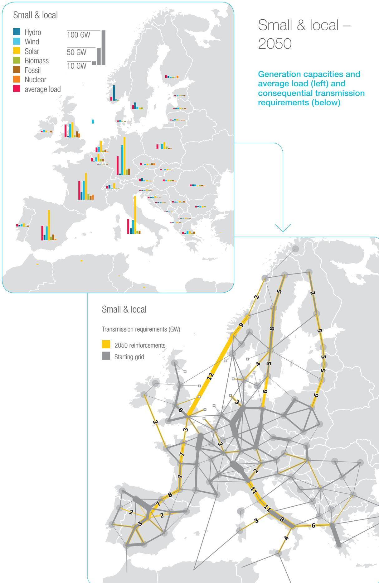
Figure 12 A: Transmission requirements identified in scenario *Small & local* (GW)
