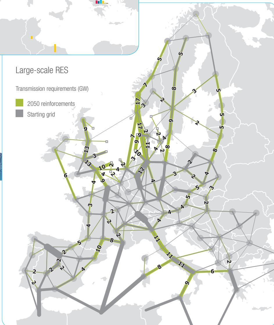
Figure 12 E: Transmission requirements identified in scenario *Large-scale RES* (GW)
