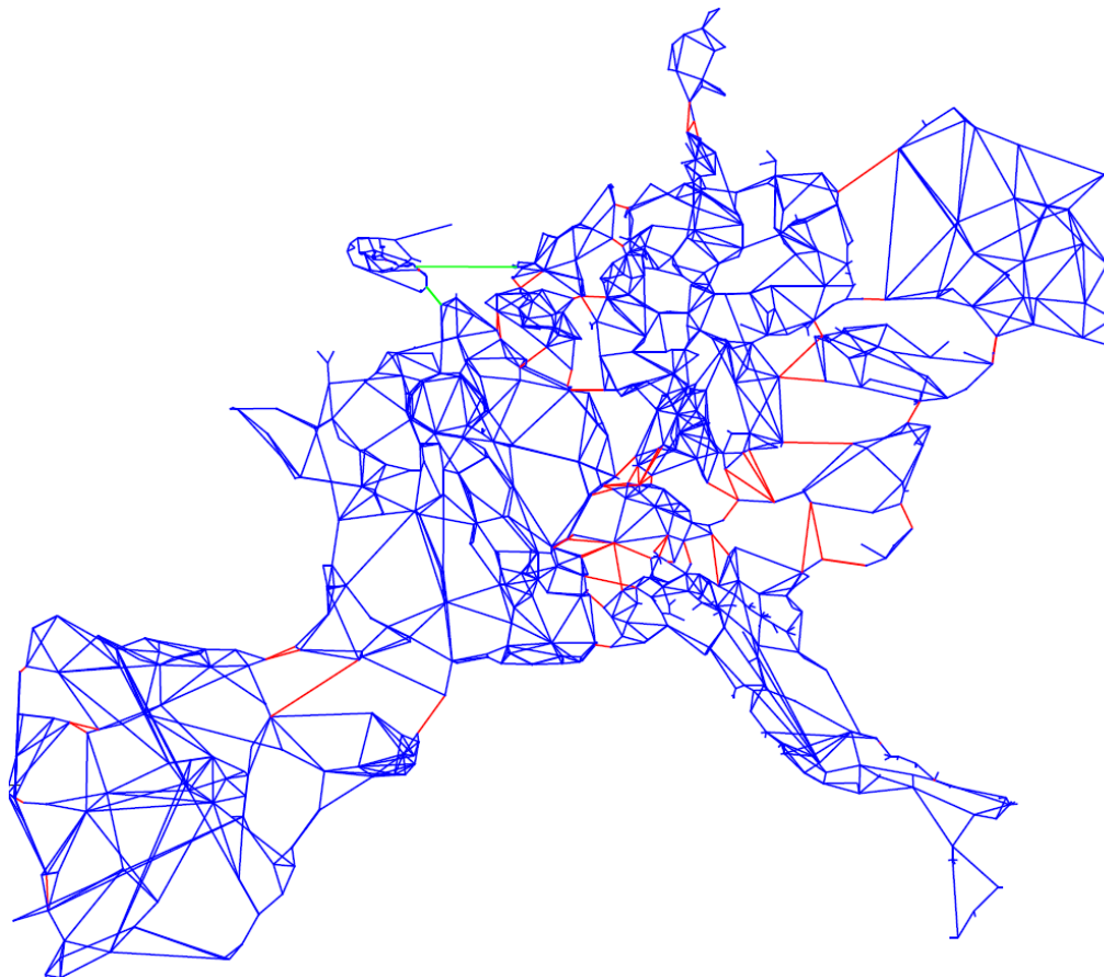
Figure 3 – Test case: initial nodal grid with 1025 nodes (HVDC links in green, AC interconnection lines in red)
