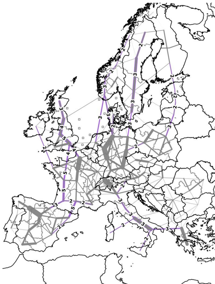
Figure 3: Grid reinforcements proposed for 2040 in addition to the projects considered in the TYNDP 2014
