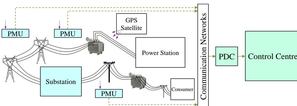
Figure 38: The deployment of PMUs in Wide Area Monitoring Systems
