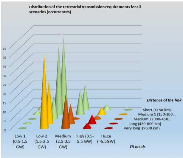
Figure 14: Distribution of the transmission requirements for all scenarios (terrestrial)
