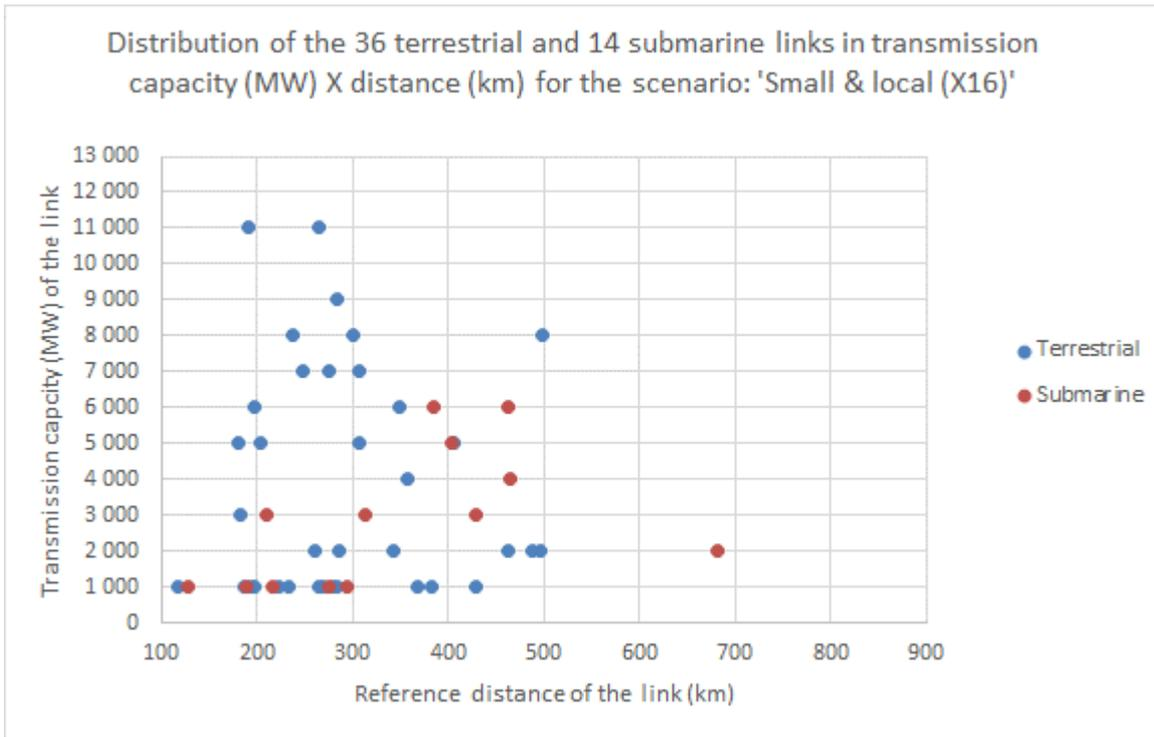
Figure 12: Distribution of the 50 links with non-zero TR for “Small and local” scenario
