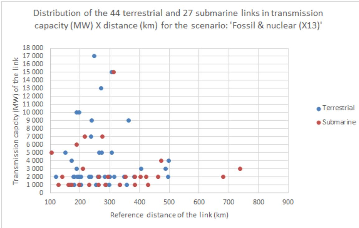
Figure 11: Distribution of the 71 links with non-zero TR for “Fossil & nuclear” scenario
