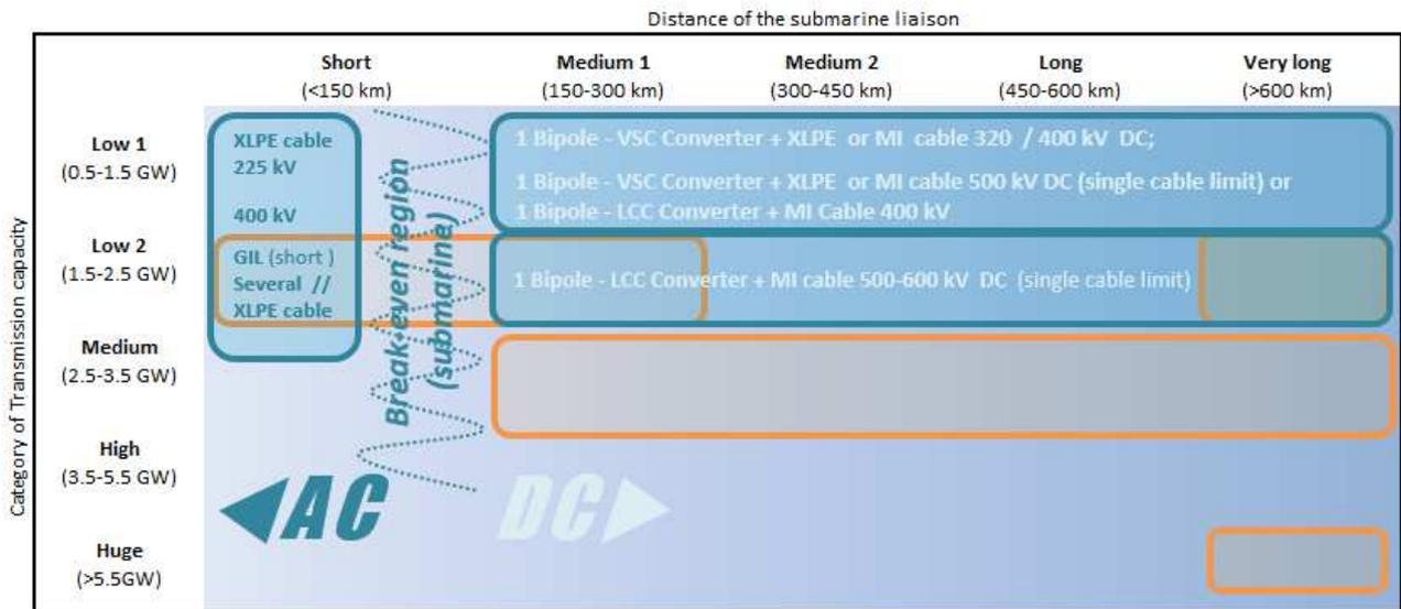
Figure 25: RD&D gap analysis: submarine needs (orange cells) compared to available technology options (blue cells)
