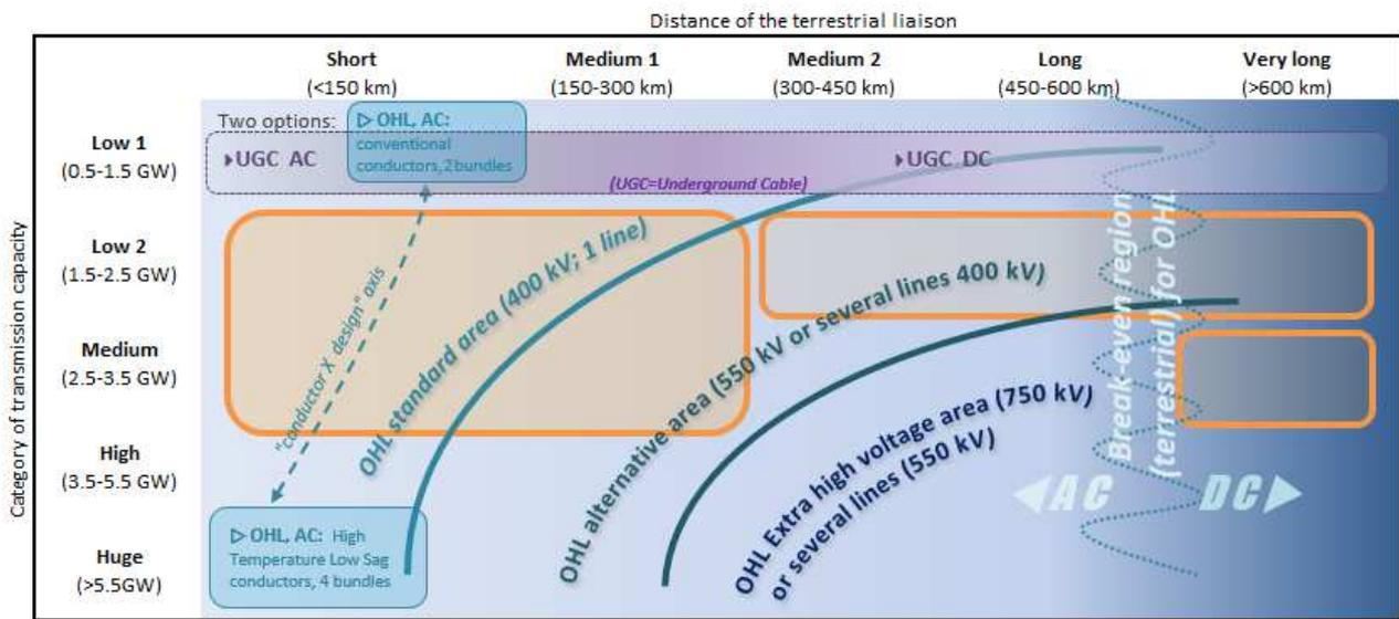
Figure 24: RD&D gap analysis: terrestrial needs (cells in orange colour) compared to available technology options (various grades of blue, from the more conventional to the less conventional)
