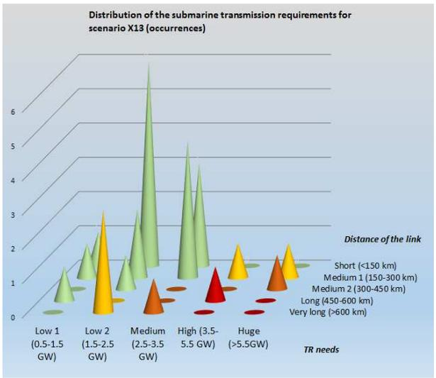
Figure 19: Distribution of the terrestrial and submarine requirements for the scenario “Fossil & nuclear” (X13)
