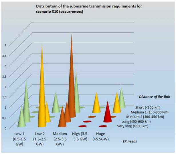
Figure 18: Distribution of the terrestrial and submarine requirements for the scenario “Big & market” (X10)
