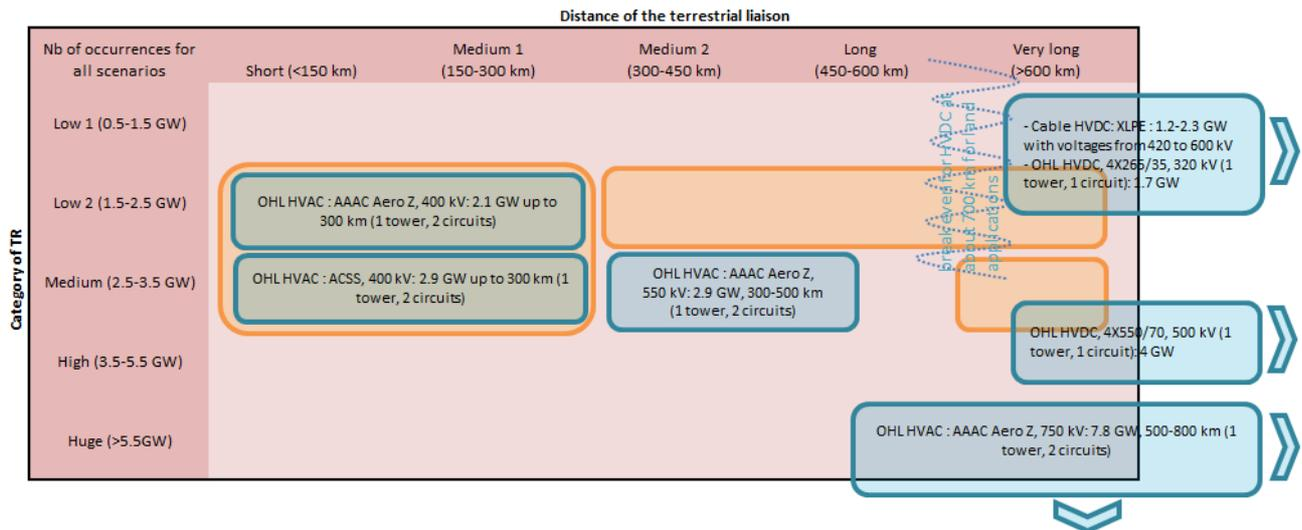
Figure 23: The technological options used in WP2 (in blue colour) compared to the needs (in orange colour) – terrestrial liaisons only
