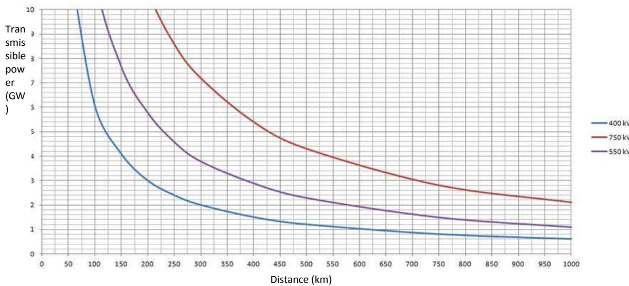
Figure 8 : Influence on maximum transmissible power over distance for different configurations of AC OHL (upper figure: two bundles per circuit; lower figure: four bundles per circuit)
