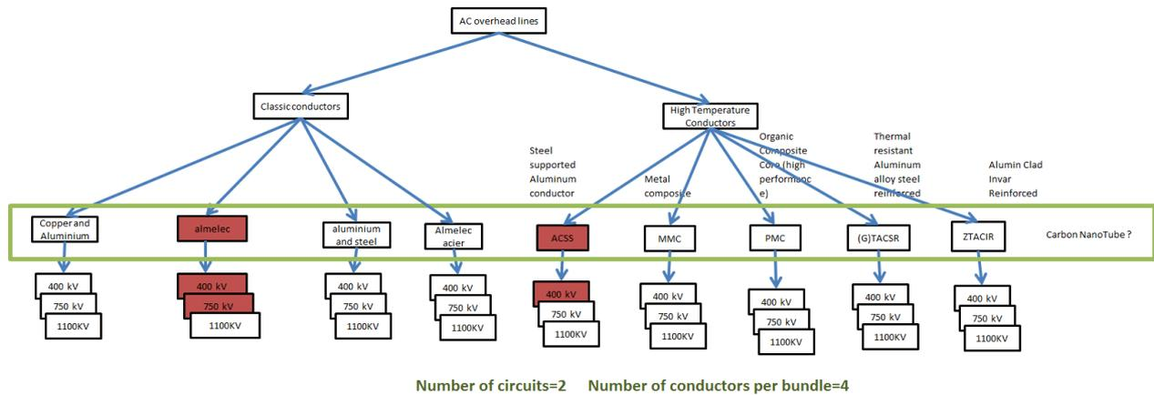
Figure 26: The e-Highway2050 selection among all conductor options for HVAC OHL
