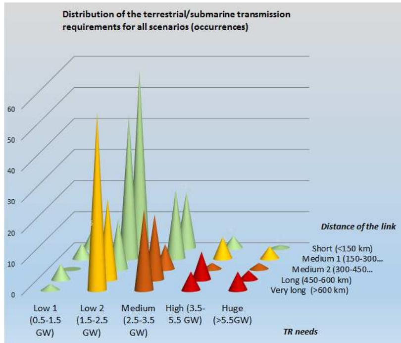
Figure 13: Distribution of the transmission requirements for all scenarios (terrestrial and submarine)
